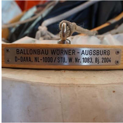
Fig.2: Marking on the envelope: stainless steel plate on the clamping ring of the appendix
