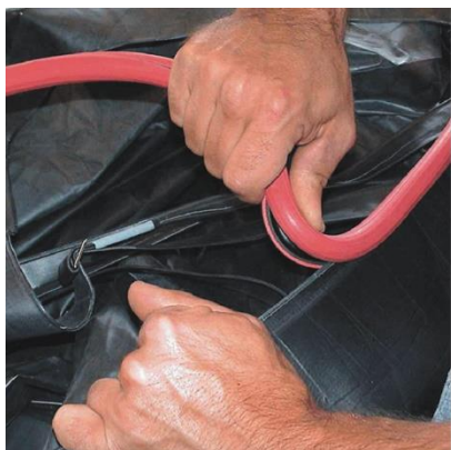
Fig. 11: Fitting the edge protection
