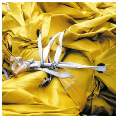
Fig. 8: Holding down patch
